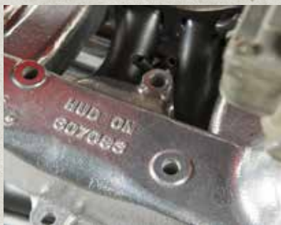
Some odd corrosion has occurred on the intake manifold and the 'S' in HUDSON has mysteriously disappeared. There was some bad corrosion on the inside edge of the intake that required repairing using plasma-spraying technology
