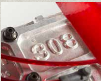
The head is from Clifford and is much thicker and beefier than the factory original with better coolant passages, higher compression and a relocated sparkplug
