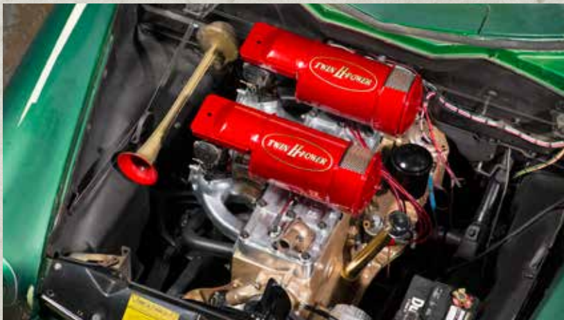
There is nothing better for Hudson fans than popping the bonnet and seeing the Twin H-Power induction sitting on top of the mighty flathead six. Tony's is more fancy than most!
