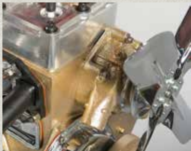
Lots of effort went into getting the paint finish durable and sparkly – gold base, lots of metallflake, then buried in clear. The manifolds and head have all been HPC coated and everything else chromed
